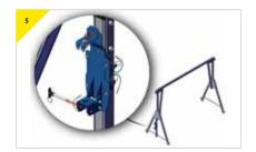
Prepare the bracket to recieve the device, making sure all the bolts for the bottom connector have been tightened. Remove the bolt from the bottom connector and loosen the top connector.
