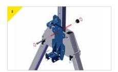
Re-align bracket and insert supplied M12 top bolt and secure.
