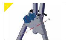
Remove bottom bolt from trap plate, and swing bracket into position.
