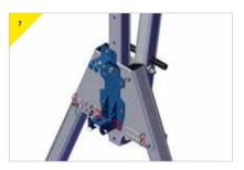
Reassemble bracket, ensuring all bolts for the bottom connector have been tightened and secured.
