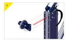
> Present the sheave bracket to the top of the column.
