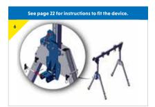
Prepare bracket to receive device, make sure all bolts for the bottom connector have been tightened. Remove pin from bottom connector and loosen top connector
