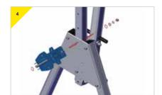
Present bracket to trap plate, insert and secure M16 top bolt supplied with bracket.
