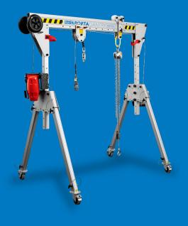
The dual-functional **PORTA**GANTRY **PAPIDE**<sup>\*</sup> was the ideal solution for utility supplier Stadtweke Elmshorn. They required fall protection for at least 2 workers who need to enter shafts via fixed ladders while also needing to lift and carefully replace 880lb pumps.
