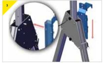
Offer up bracket using keyhole slot, hook and push bracket down into place and tighten the bolt to secure.
