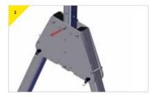
Loosen the top bolt without removing.
