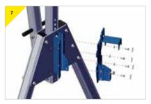
> Re-assemble the bracket to the plate.
