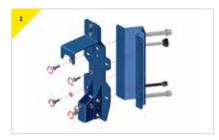
Before attaching the bracket to the device, dissemble the bracket.
