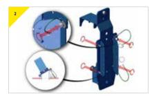
Adjust the width of the wings to 3" (76.2mm) and fit the bracket onto the column.
