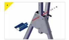
Present the bracket to the trap plate, insert and secure the M16 bolt supplied with the bracket.
