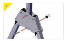
> Remove the bottom bolt and loosen the top bolt.
