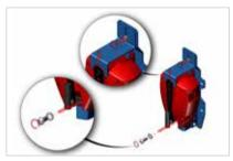
Insert the bottom bolt to secure the device into position. Adjust the top connector in the suitable position and secure by tightening the bolt.
