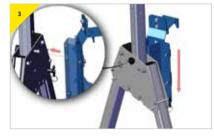
Offer up bracket using keyhole slot, hook and push bracket down and tighten the bolt.
