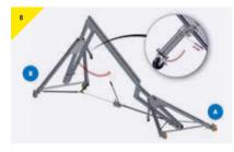
Once A-Frame B has met the beam, the wheel assembly can now be folded away. Use the pin provided to retain the position.
