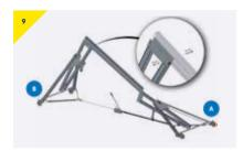
Secure A-Frame B and beam by placing the bolt provided with the A-Frame.
