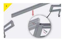
> Place the beam on the A-Frames as per the usual gantry assembly.
