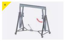
> Erect A-Frame A with the pulling device. Once A-Frame A is in position, the wheel assembly can now be folded out of the way. Use the pin provided to retain the position.
