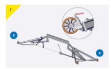
Put the brake on A-Frame A and erect A-Frame B with the pulling device.
