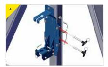
> Insert pins provided to secure bracket to section.
