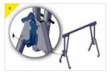
Prepare the bracket to receive the device and remove the pin from the bottom connector and loosen the top connector.
