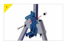
Insert the supplied M12 top bolt and secure.
