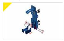
Before attaching the bracket to the device, dissemble the bracket and remove the the bottom connector.
