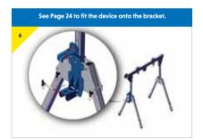
Prepare the bracket to recieve the device, make sure all the bolts for the bottom connector have been tightened. Remove the pin from the bottom connector and loosen the top connector.
