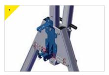
Re-assemble the bracket to the plate. Make sure all the bolts for the bottom connector have been tightened.
