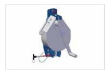
Insert the bottom pin to secure the device into position, making sure the pin is fully engaged. Adjust the top connector in the suitable position and secure by tightening the bolt.
