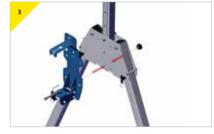
Present the bracket to the trap plate, insert and secure the M12 bolt supplied with the bracket.
