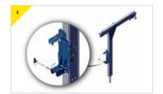
Prepare the bracket to recieve the device, make sure all the bolts for the bottom connector have been tightened. Remove the bolt from the bottom connector and loosen the top connector.
