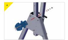
Present the bracket to the trap plate, insert and secure the M16 top bolt supplied with the bracket.
