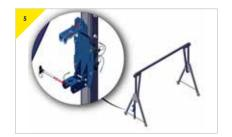
Prepare the bracket to recieve the device, making sure all the bolts for the bottom connector have been tightened. Remove the bolt from the bottom connector and loosen the top connector.
