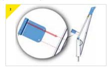
> Present the bracket to the backstay, ensuring that the correct holes line up ready to secure.
