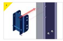
Present the bracket to the TDAVIT column, ensuring that the correct holes line up ready to secure.
