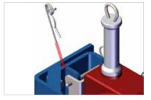
Insert the pin provided the secure the pin in place.
