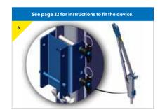
> Bracket is ready to receive the device.
