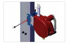
Insert the pin supplied with the bracket as shown to secure the device in place.
