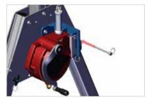
Insert the pin supplied with the bracket as shown to secure the device.
