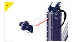
Presen the sheave bracket to the top of the column.
