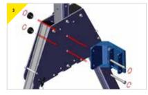
Present bracket to trap plate, insert and secure M12 bolt supplied with bracket.
