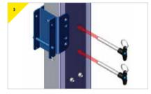
Insert the pins that have been provided with the bracket.
