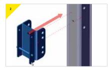
Present the bracket to the winch column, ensuring that the correct holes line up ready to secure.
