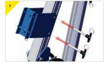
Insert the pins that have been provided with the bracket.
