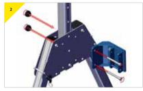
Present bracket to trap plate as shown, use trap plate centre holes to insert and secure both M12 bolts that have been supplied with the bracket.
