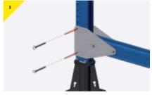
> Secure the Davit using the detent pins provided.
