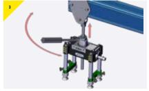
Engage the ratchet and apply the load. Once the required loading has been achieved, hold the load for the amount of time determined by the local authority regulations. De-load by rotating the ratchet in the opposite direction.
