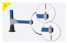
Depending on the device used for testing the socket, pull or push up the Test Davit using the necessary equipment to the required load. Once the Davit has been assembled in place it is ready for a device to be attached to the shackle point or clevis pin to begin the test.
