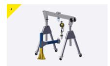
Fit the chain block and the loadcell in between the trolley on the gantry and the shackle on the test davit.
