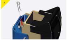
> Secure the pin using the R-Clip provided.
