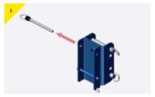
> Remove the pin from the bracket.
