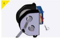
> Secure the device using the pin.
