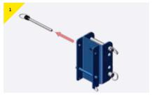
> Remove the pin from the bracket.
