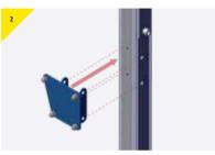
> Remove the pins and present the bracket to the winch column, aligned to the holes as shown.
