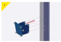
> Remove the pins and present the bracket to the column, aligned to the holes as shown.
