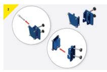
Disassemble the bracket by removing the pins, bolts and separating the pieces.
