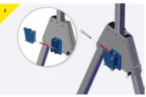
Reassemble the bracket using the pins provided as shown. First the lower pin and slide into place and secure with the top pin.
