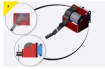
> Adjust the position by tightening the hex bolts.
