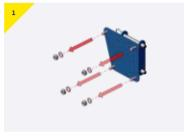
> Remove the washers and nyloc nuts from the bracket.
