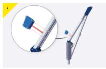
> Remove the pins and present the bracket to the backstay, aligned to the holes as shown.
