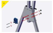
Present the bracket to the trap plate as shown, secure both M12 bolts through the correct holes as shown.
