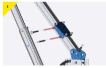
> Insert both pins to ensure the bracket is securely attached.
