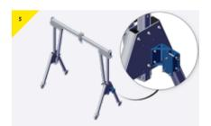
The following instructions detail the assembly of the IKAR PLW bracket [US-RAWB004200] for the PORTAGANTRY'.
