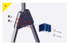
Present the bracket to the trap plate and secure with the M12 bolts supplied. Ensure to align the lower bolt to the same hole as the bolt was just removed from.
