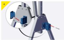
Reassemble the bracket using the pins provided as shown. First the lower pin and slide into place and secure with the top pin.
