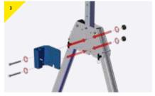
> Present the bracket to the trap plate and secure in the central holes using the M12 bolts supplied.
