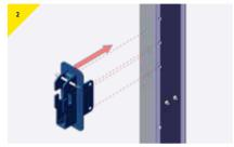
> Remove the pins and present the bracket to the column, aligned to the holes as shown.
