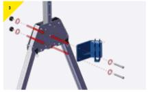
> Present the bracket to the trap plate using the centre holes, securing with the M12 bolts.
