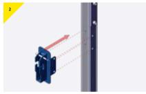
> Remove the pins and present the bracket to the winch column, aligned to the holes as shown.
