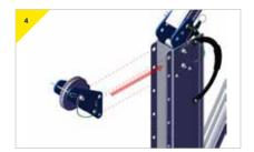
Presen the sheave bracket to the top of the column.
