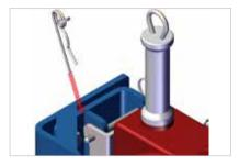
Insert the pin provided the secure the pin in place.
