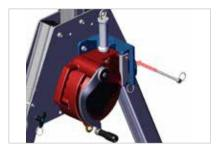
Insert the pin supplied with the bracket as shown to secure the device.
